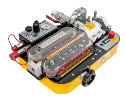
The C-1900 JetStream has been designed to provide maximum cable protection, combined with the performance and reliability of hydraulic drive. The profiled double drive belt system is driven by single 32cc hydraulic motor, powered by the proven C-1203-F power pack.
